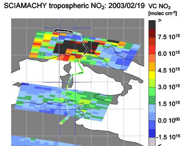
Fig. 4. SCIAMACHY and AMAXDOAS tropospheric vertical column, plotted in the same colour scale.
