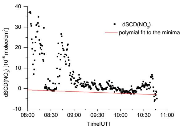
Fig. 2. Differential slant column densities of NO<sub>2</sub> and a polynomial fitted to the minima. The polynomial is subtracted afterwards to retrieve the tropospheric SCD.
