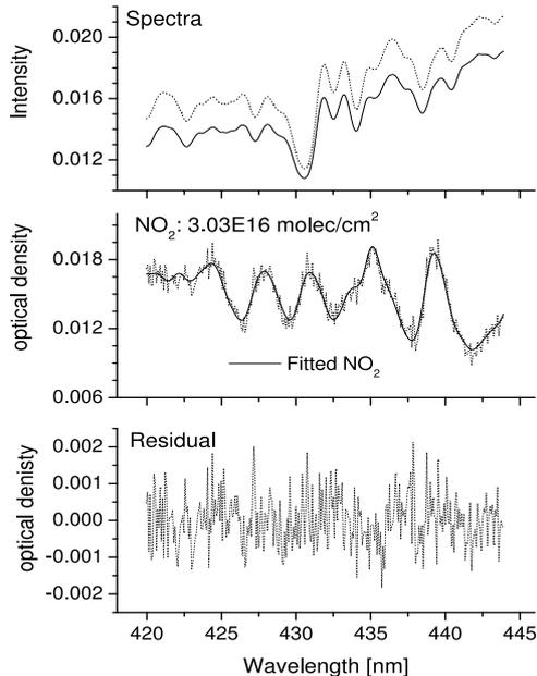
Fig. 1. DOAS-fit for NO<sub>2</sub> of a Nadir spectrum. The spectrum was taken 19 Feb. 2003 at 8:14:30 close to Zürich. The reference was taken 30min later over the Alps.
